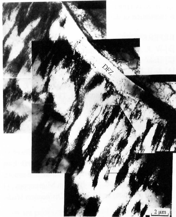
Fig. 7 Dislocation substructure observed in the specimen annealed at 773 K and fatigued at 24 MPa for 10^{10} cycles.
