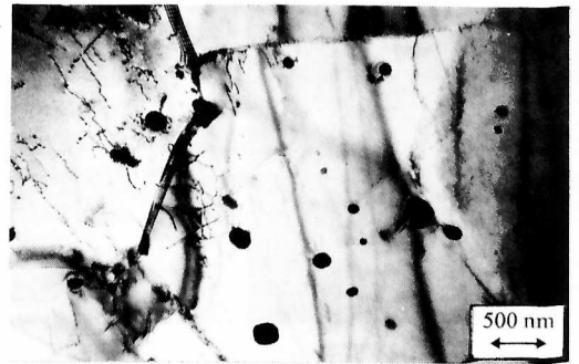
Figure 4 TEM micrograph showing the low dislocation density in the nugget zone of friction stir welded AA 6082.
