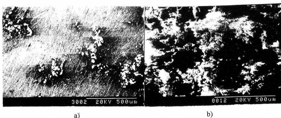
Fig1 Scanning electron micrograph ( \times 100 ) of alloy LC9 after immersion of 10 days in: a) Solution 1; b) Solution 2
