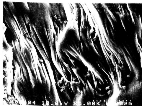
Fig.6 SEM microstructure of specimen surface near of the fracture surface and the strain rate of 0.25s-1 at 873k.
