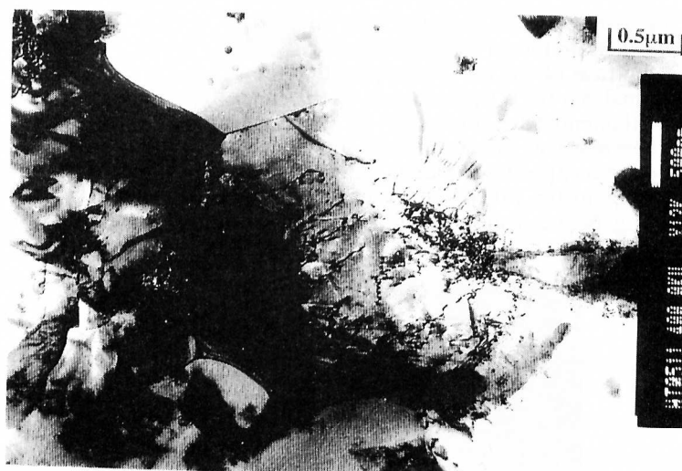
Fig.8 TEM microstructure of as-heated SiCp/6061 Al alloy composite.
