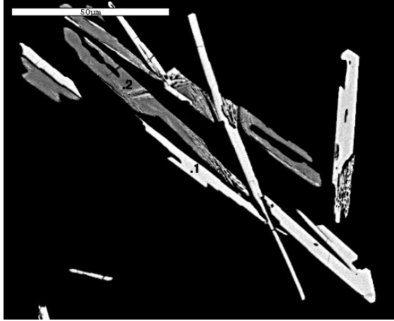
Figure 7: Back-scattered image of SEM showing flake-like particles with different compositions.
